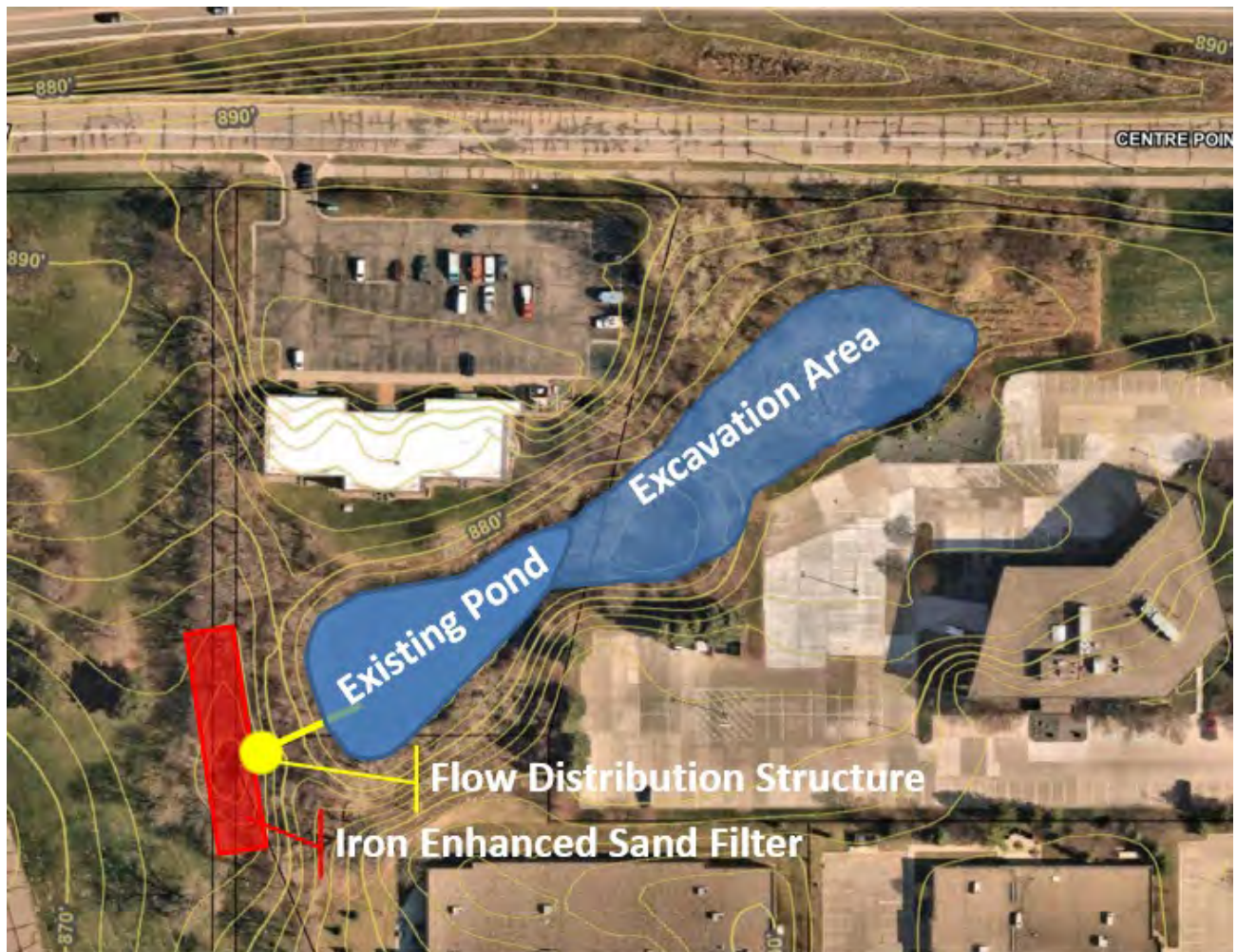
Figure 5-4 Conceptual Design of Stormwater Pond 2 Enhancements
